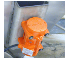
Vibratory Hopper For intermittent use to promote flow into the conveyor inlet.
