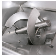
Ribbon Agitator Ideal for sluggish materials that may bridge or rathole.
