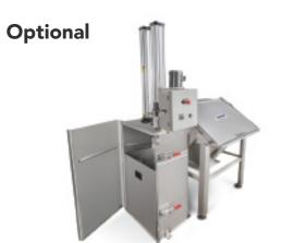
Keep areas surrounding your operation clear of debris and dust with a bag compactor. Hapman compactors attach to the side of your bag dump station through an access port in the station's side wall. Empty bags pass easily into the compactor, so dust does not have an opportunity to leave the station.
