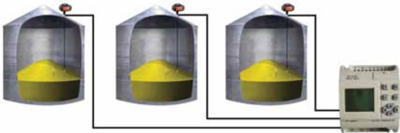
The SmartBob AO features a direct 4-20 mA analog output.
