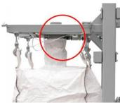
Venturi Bag Inflation Inflates the bag to maximize capacity by removing folds and creases in the bag prior to filling.
